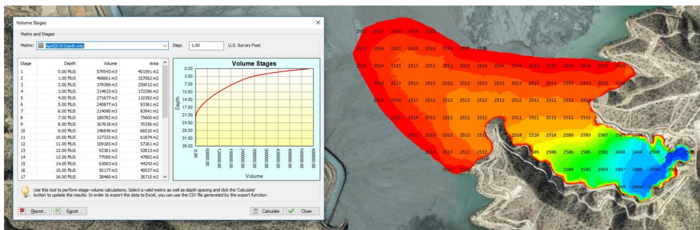
Figure 1, Tailings pool bottom elevations and water volume versus stage – extrapolated to the beach.
