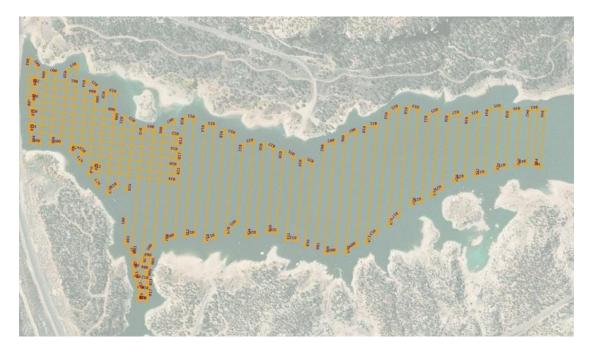
The routes were designed to provide adequate coverage to determine large scale features but ensure the surveys were completed in one day per site. The GNSS used was the CEESCOPE LITE<sup>™</sup>
