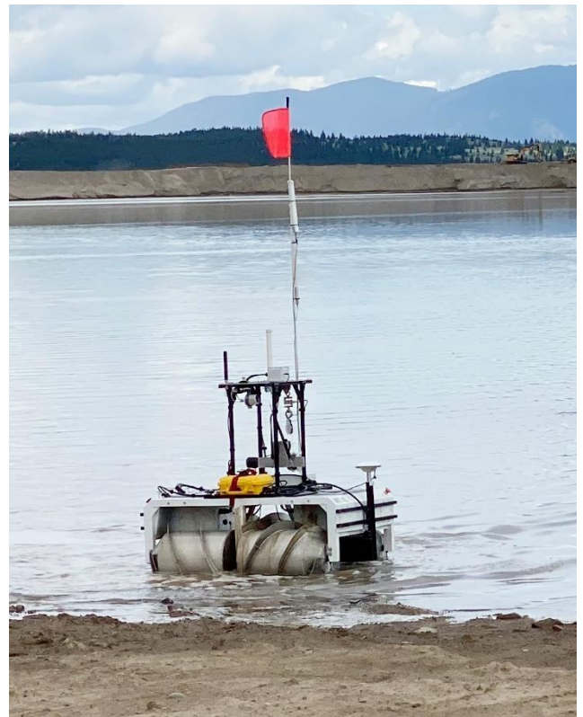
HELIX with CEE ECHO™ 33/200 kHz echo sounder.
