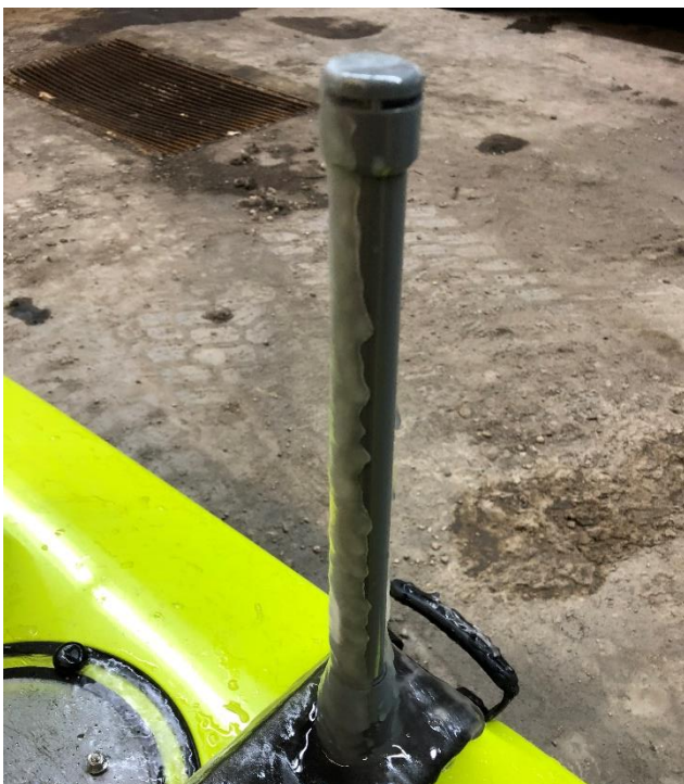
Ice buildup only on the front side of antenna.
