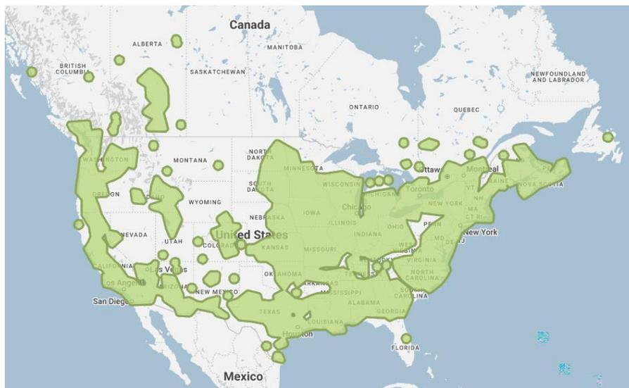
After logging in to the service, the user can select to receive corrections from a “drop down” list of nearby base stations, or for “Virtual Reference Station” (VRS) services, the closest base stations are used in combination to compute the error that would be expected at the exact position of the receiver, potentially improving accuracy as the receiver moves around. Some network RTK services are available free of charge, with users able to connect to single base stations operating locally.
