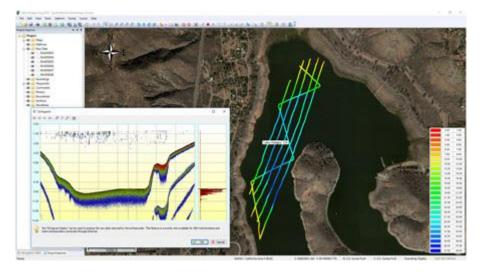
**Dual Frequency Operation:** Using a dual frequency transducer to obtain results related to sedimentation is only properly managed with hydrographic acquisition software to understand the context of the high and low frequency data, although it is possible to use dual frequency with a limited scope when operating in the land survey approach.
