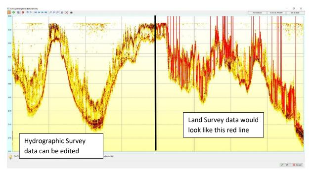
Accuracy: The CEE ECHO<sup>™</sup> and CEESCOPE<sup>™</sup> mesh GNSS and depth data and apply a precise millisecond time stamp used in the software to exactly position soundings. Latency errors are eliminated. These echo sounders output data at up to 20Hz, leading to far greater detail and significantly more resilience – retaining good data even after substantial thinning during editing.
