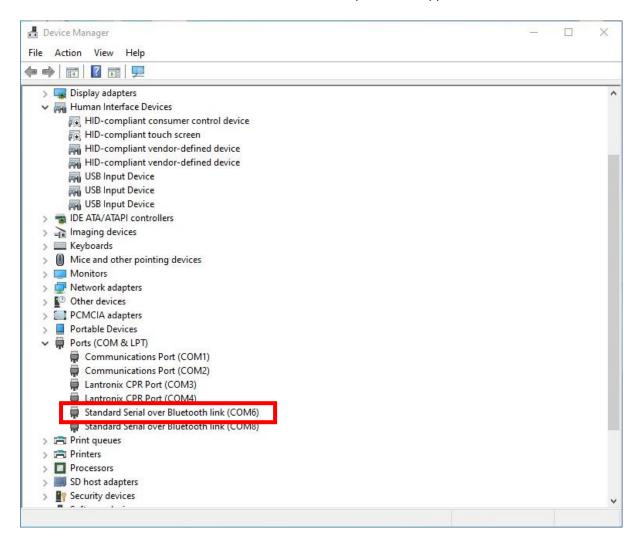
In order to test the Bluetooth data link, TeraTerm may be used to display the data available on COM6.
