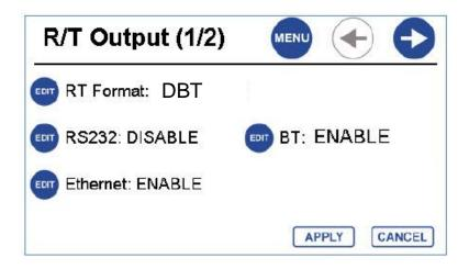
For typical applications using GNSS software, it is appropriate to select DBT (depth below transducer). This will report the depth with no draft included, allowing the transducer to GNSS antenna offset to be entered into the GNSS software as with a normal rod height. Alternatively, DBS (depth below surface) can be used which will incorporate the echo sounder draft offset (**ES 1/6 m**enu). Most other output formats will not be recognized by GNSS software.
