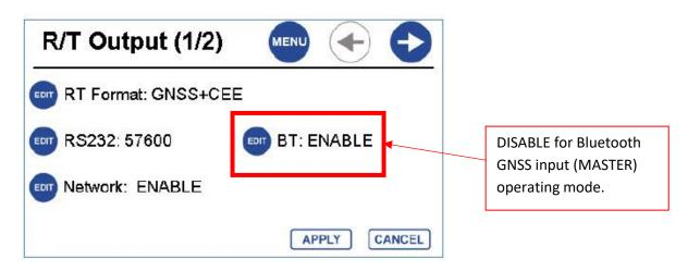
To establish an incoming Bluetooth data connection, first select BLUETOOTH\_MASTER on **System** (1/8) menu. The "BT Password" is the password needed to access the connected GNSS device so this must match what is required by the GNSS receiver. The password is set by pressing EDIT for the "BT Password".
