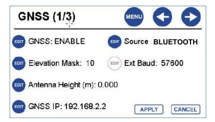
NOTE: Some CEE ECHO firmware versions will NOT display the BLUETOOTH source option on the GNSS (1/3) menu unless the Real Time (R/T) Output (1/2) menu shows Bluetooth output is DISABLED.
