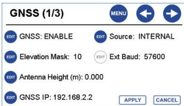
GNSS menu indicating CEESCOPE-R™ GNSS receiver IP address.
