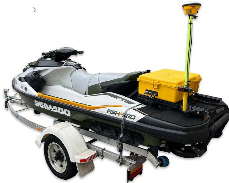
CEE-JET 1600™ Survey system installed on SeaDoo FishPro PWC (2022 model).
