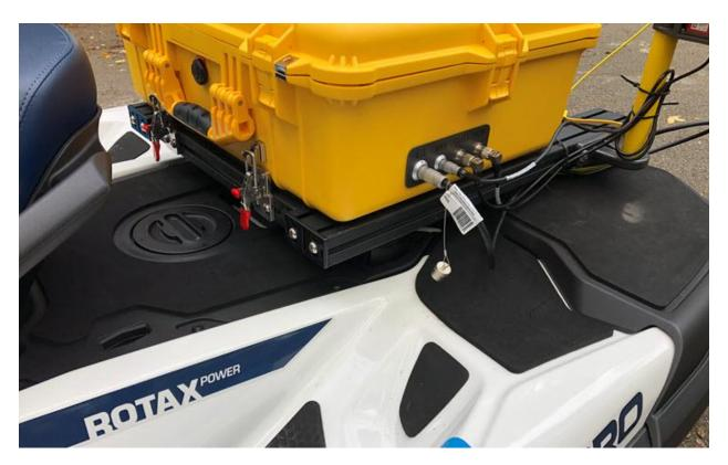
Likewise, for the 200kHz transducer the special attachment pod screws into existing bolt holes. The transducer placement was determined after sea testing to ensure maximum protection against aeration artifacts. Indeed, even in rough water with high pitch and roll movements the sonar data are surprisingly clean and free of spiking artifacts.
