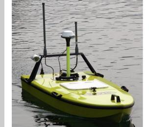
The Dynautics SPECTRE autopilot system integrated into the CEE-USV now may be operated through HYPACK. With no requirement for any other operating interface, all route planning and uploading may be handled within HYPACK. Simply create the line plan and the driver sends the lines as waypoints to the USV - ready to survey! Watch the video below to see how it works.
