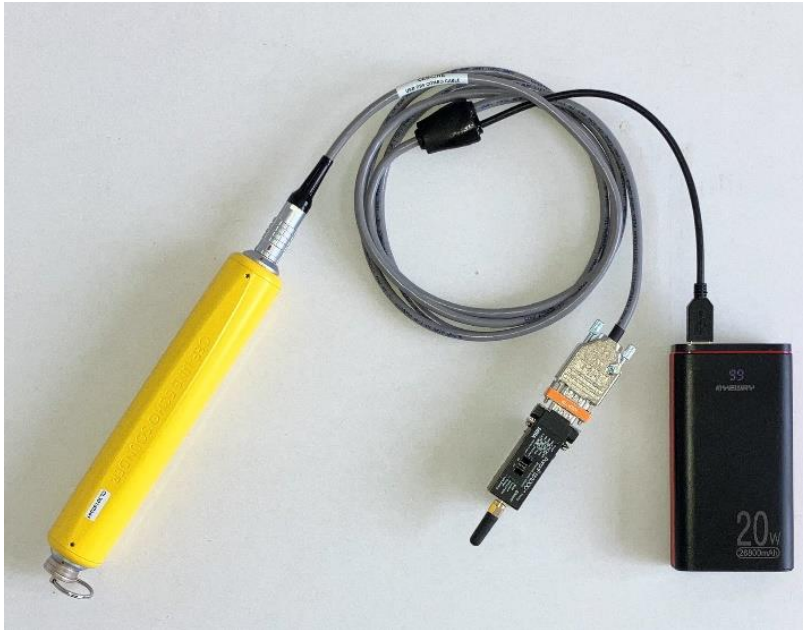
Figure 2. CEE-LINE with external SENA Parani SD1000 Bluetooth Module and USB Power Pack.
