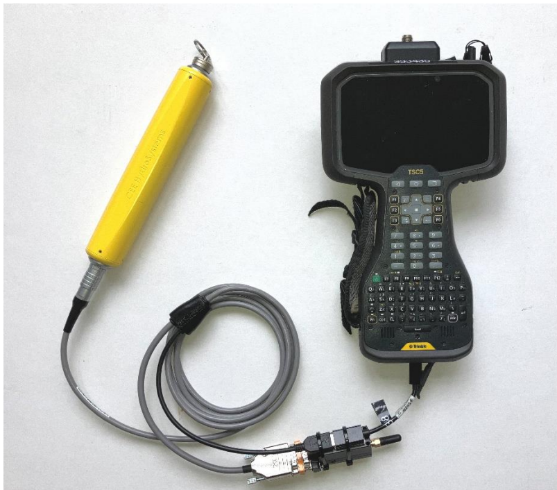
Figure 1. CEE-LINE with external SENA Parani SD1000 Bluetooth Module powered by TSC5.
