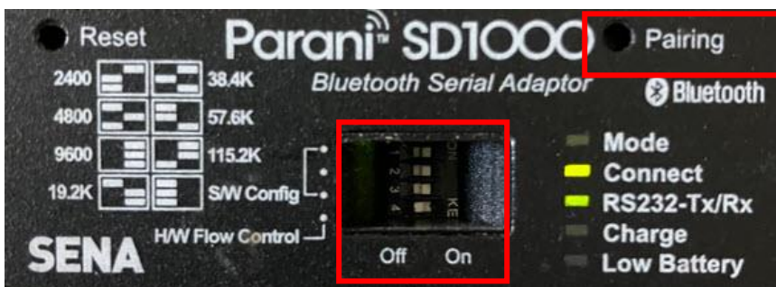
Figure 3. SENA Parani SD1000 showing dip switches and pairing button.
