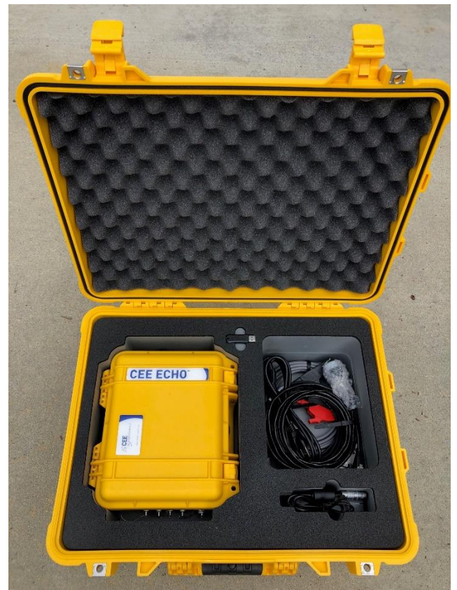
CEE ECHO™ portable survey echo sounder kit.
